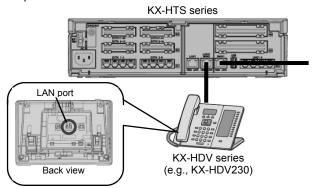
2. KX-HDV series will be registered to KX-HTS series automatically. Confirm that an extension number (e.g., 101) is displayed on the LCD of KX-HDV series.
